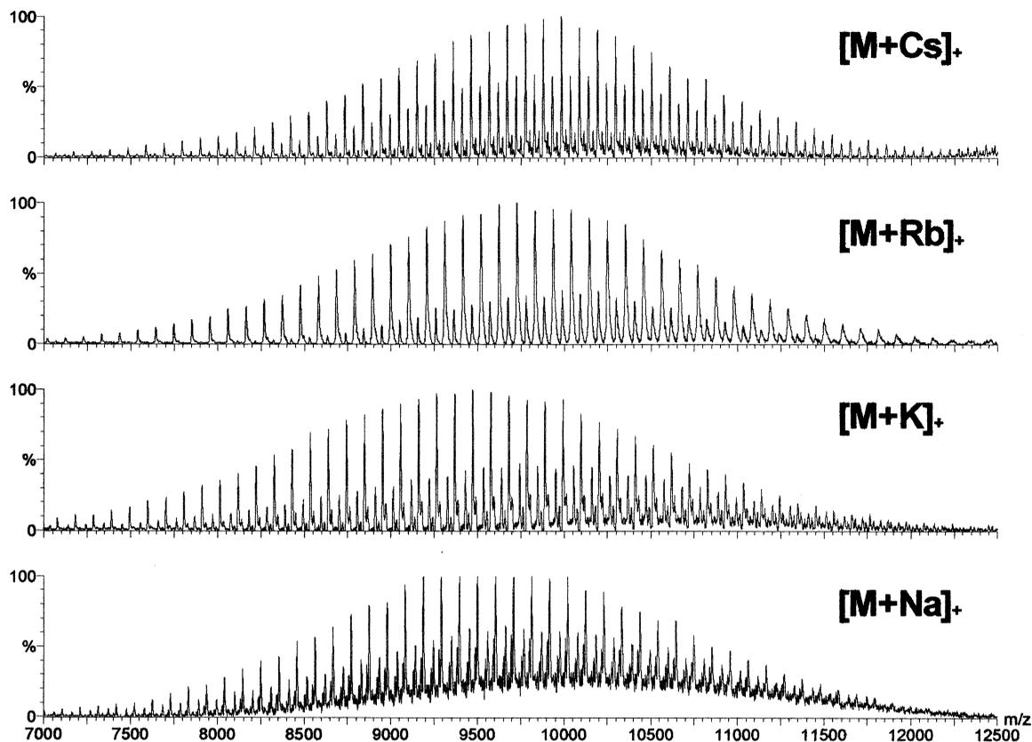
Fig. 5. Electro spray spectra obtained in an orthogonal acceleration time-of-flight (oa-TOF) mass spectrometer from poly(styrene) 9850, using alkali metal cations for ionisation.
