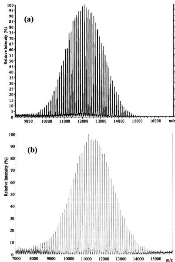
Fig. 1. (a) FD-MS and (b) MALDI-TOF spectra of a narrow polydispersity poly(styrene) sample with an average molecular weight of approximately 12.5 kDa.
