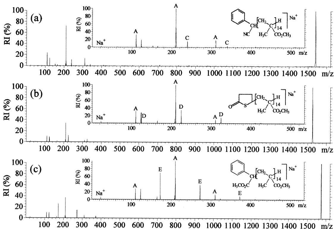
Fig. 7. MALDI-CID spectra from PMMA samples with different initiating end groups (see text for description of fragmentation), obtained in a hybrid sector-oa-TOF mass spectrometer. The A, C, D and E series of peaks allow information on the masses of the end groups to be inferred.
