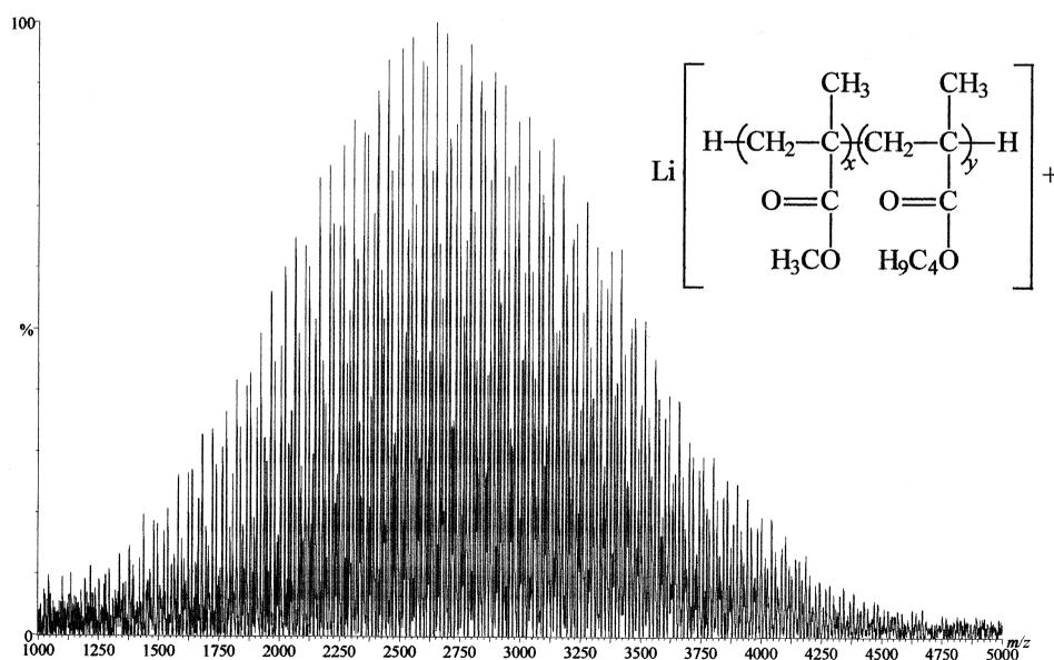
Fig. 3. MALDI-TOF spectrum of a block methyl methacrylate/butyl methacrylate (MMA/BMA) copolymer that was generated by means of group transfer polymerisation (GTP).
