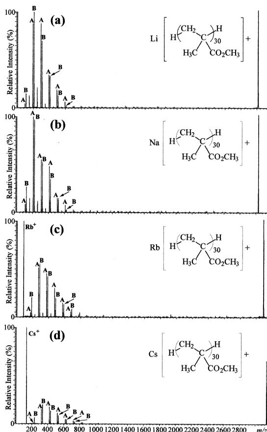
Fig. 10. MALDI-CID spectra of the 30-mer of poly(methyl methacrylate) (PMMA) with ionisation by addition of varying alkali metal salts, obtained in a hybrid sector-oa-TOF mass spectrometer. The A and B series of peaks allow information on the masses of the end groups to be inferred.
