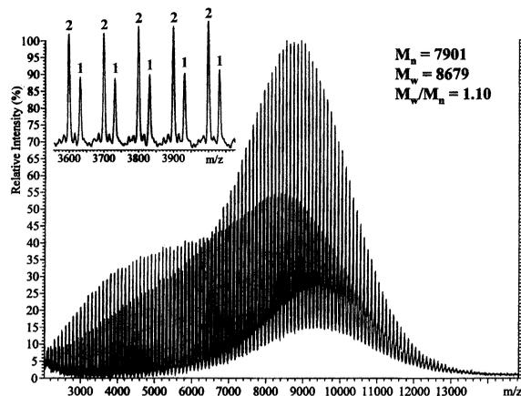
Fig. 2. MALDI-TOF spectrum of a poly(methyl methacrylate) (PMMA) sample [that was generated by means of group transfer polymerisation (GTP)], indicating that species with two modes of termination are present.
