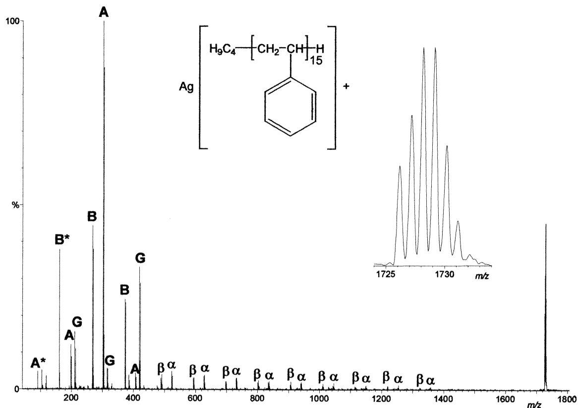
Fig. 9. MALDI-CID spectrum of the 15-mer of a poly(styrene standard), obtained in a hybrid quadrupole-*oa*-TOF mass spectrometer. The fragmentation pattern (namely the A and B series) enables end group information to be inferred.
