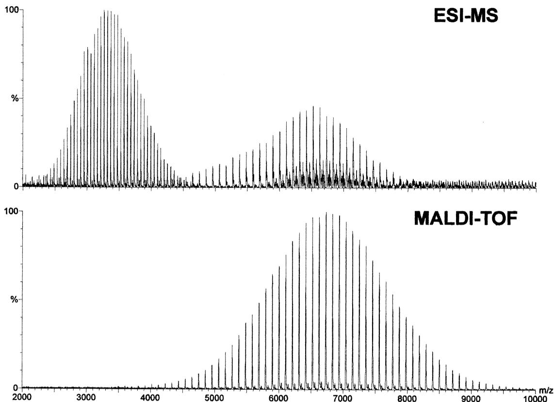
Fig. 6. Electropray (obtained in an oa-TOF mass spectrometer) and MALDI-TOF spectra obtained from poly(styrene) 7000, using silver ions as the cationisation agent.
