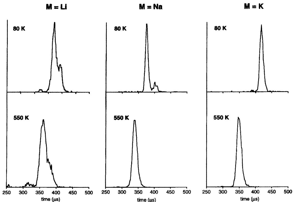
Fig. 12. Arrival time distributions for lithiated, sodiated and potassiated trimers of poly(ethylene terephthalate) (PET) at 80K and 550K.
